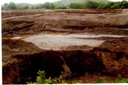
Figure: (7). Open-pit mining site (No. P 1 -13) in Kyauktaga-Legy Agglomerate unit, for the production of natural pozzolan.
